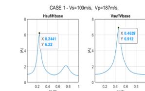
Figure 5: Amplification Function (case 1)
