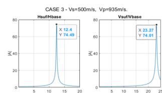
Figure 11: Amplification Function (case 3)
